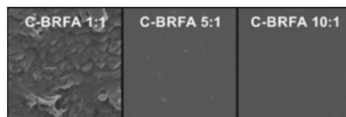
The micromorphology of C-BRFA at different ratios of microcellulose versus BRFA characterized by Scanning Electron Microscope
