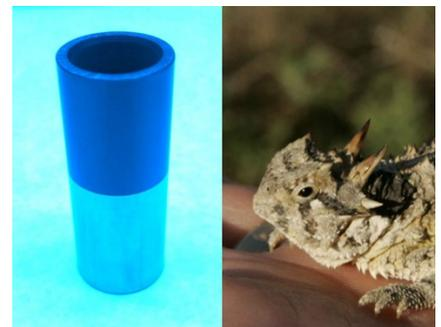
The developed method is suitable to treat parts under friction like this metal shaft whose surface structure emulates some structures found in nature. The dark blue upper part of the shaft has been structured to ensure adequate lubricant wetting and transport.
