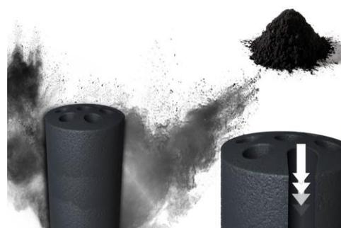
The integral carbon monoliths thus obtained are extremely useful in processes that involve solid-basic catalytic reactions, such as, the control of environmental contamination, the selective hydrogenation of NO<sub>x</sub>, the catalyzed oxidation of volatile organic compounds and the biodiesel synthesis and methane reforming.
