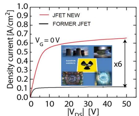
Main examples of environments where electronic devices should present radiation hardness. Comparison between density Current between the new developed and former JFET device.
