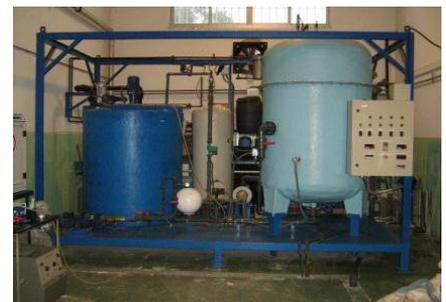
Anaerobic digester for biogas production.
