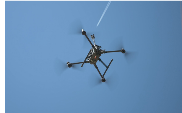
Meteo-Drone taking meteorological measurements of the atmosphere.
