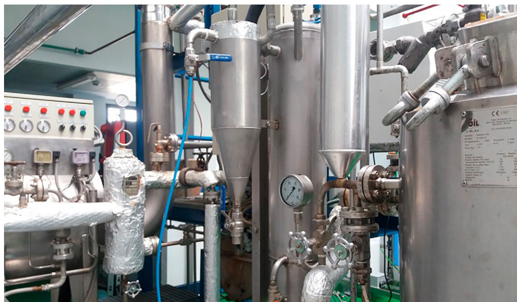
Phytochemical pilot plant heat treatment reactor and laboratory chromatographic columns, developed for the extraction and purification of comselogoside from olive oil by-products.
