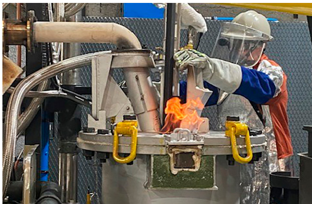
Submerged arc pilot plant for the recovery of critical and strategic metals.
