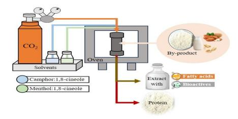
Design of a plant which uses supercritical CO2 and eutectic mixtures applied to by-products from the almond and peanut beverage production process. Obtaining extracts rich in bioactive compounds and protein-rich extracts.
