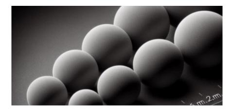
Highly spherical, monodisperse particles made of titanium oxide can be synthesised in a sub and micrometre range under very mild conditions in a facile synthesis using commercial reactants. Applications in catalysis and photonics
