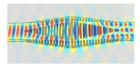
New modal conversion architecture comprising two Yjunctions facing each other, with a subwavelength metamaterial structure in between them.
