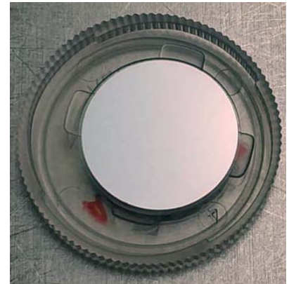
Ultraviolet filter type surface of a part after being coated using the developed thermal source
