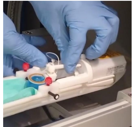
Device mounted in a RMN scanner bed to be used on an imaging phantom in a laboratory test.
