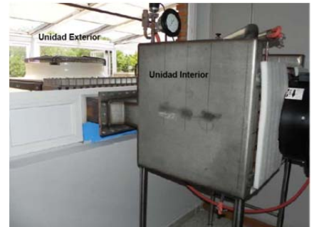
Absorption refrigeration machine prototype air-air and split installed in the testing bench
