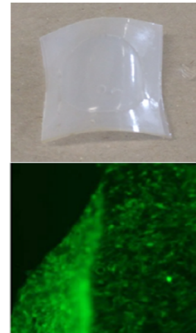
Top: nylon coated with thermosensitive hydrogel. Bottom: cell monolayer being detached by temperature decrease
